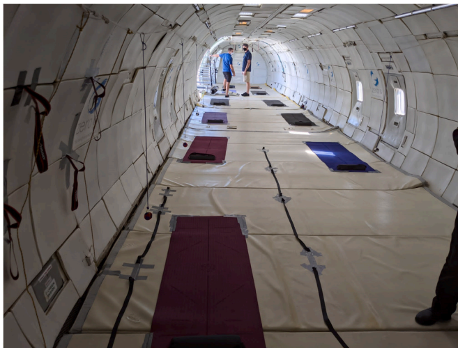
Fig. 2. The Zero-G Aircraft (left) View of the aircraft cabin ahead of Flight AA1 showing a long, white, open tube with padded walls and floor. A large door is seen on one side of the craft letting light inside, and two individuals are conversing in the background. Cables, straps, and footholds are visible duct taped to the cabin walls and floor, as well as two parallel rows of yoga mats.
