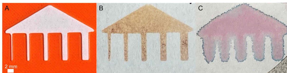
Fig. 4 (A) Sample mask made in orange plastic. (B) Paper coated with TCMS and patterned with oxygen plasma, with dye added to visualize the channels. (C) Paper coated with TCOS and patterned with oxygen plasma, with dye added to visualize the channels.
