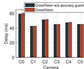
Fig. 10. Frame inference delay of CrossVision and CrossVision without accuracy guard.
