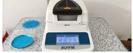
Fig. 12. The SN-DHS-16 moisture dryer for ground truth.
