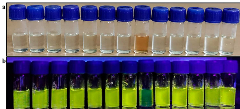
Figure 6. Photographs of luminogen (TPE-SKJ) with different anions (a) under ambient (day) light and (b) under UV irradiation (365 nm).
