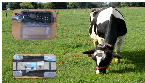
Fig. 1 Recording system used to record the acoustic signals composed of inward and outward facing microphones (a). Wired microphones were covered by an elastic headband (b) and plugged (c) into a recorder housed inside a weather proof case attached to the top side of a halter neck strap (d).
