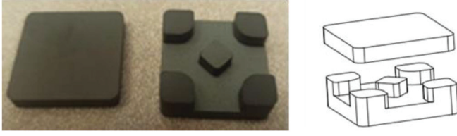
Fig. 26. Core shape of the integrated matrix auto-transformer.
