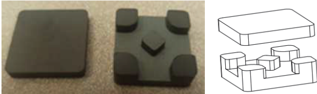
Fig. 13 The model of integrated transformer
