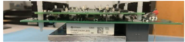
Fig. 15. Vertical structure of gate driver board design
