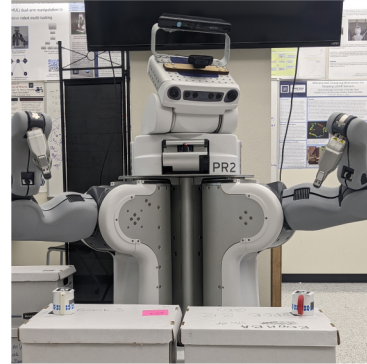
Fig. 1. This figure shows a PR2 robot picking up both of the cups in front of it. The PR2 has two arms and they are both free, so it should pick up both cups simultaneously.
