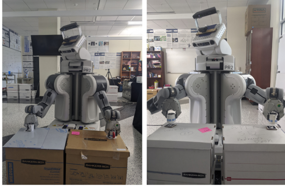
Fig. 5. These images show PR2 simultaneously running behaviors during experiment 1. The image on the left shows PR2 picking up both objects 1 and 2. The image on the right shows PR2 placing objects 3 and 4 together.
