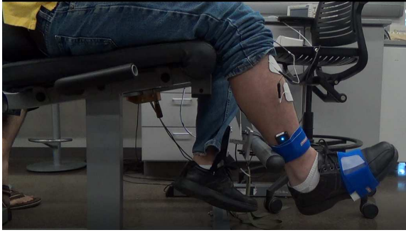
Figure 1. Seated task setup - The electrodes were placed on the TA muscle with stimulation parameters set at f = 50\text{Hz} , i = 25\text{mA} , and the pulse width was varied to determine the threshold and saturation values for ankle dorsiflexion and use them further for system identification, and the inertial measurement unit was placed on the shank and the foot.
