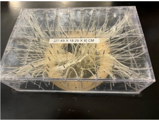
Figure 2: The low-rise model with pressure taps installed
