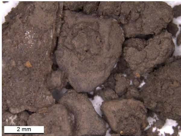
Figure 4. Optical image of undersized BFS.
