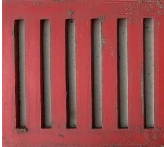
Figure 3. 3-D printed molds used to create three-point bend coupons.
