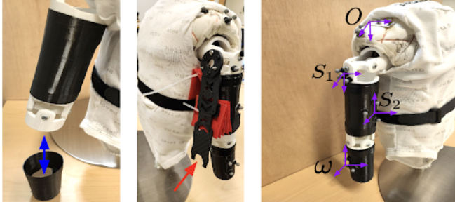
Fig. 5. (Left) Our engineered mannequin built in-house integrates 3D-printed joints and links (upper-arm and forearm) designed based on anthropometric data. The links are adjustable (easily swappable and hollow to be filled in with additive weight) to make the mannequin easily reconfigurable. (Center) Embedded supporting structure to mount one end of the shoulder flexion/extension actuator. (Right) The various coordinate systems employed in kinematics analysis and control of the overall system.
