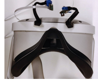
Figure 4: Hardware prototype attached to VR headset (Oculus Quest 2).
