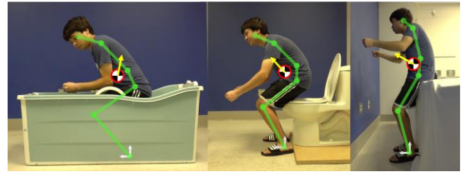
Figure 8. Human subject at the point of most difficulty (maximal muscle exertion) for three activities of daily living. Also shown is the position (red circle) and normalized velocity (yellow vector) of the center of mass of the first five body links.
