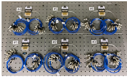
Fig. 1. Datacom HOPE kit with six packaged PICs (Chip 1: insertion loss; Chip 2: interference; Chip 3: Mach–Zehnder modulation; Chip 4: germanium photodetectors; Chip 5: ring resonators and wavelength division multiplexing; Chip 6: ring resonator modulation) covering the fundamental concepts of data communication.
