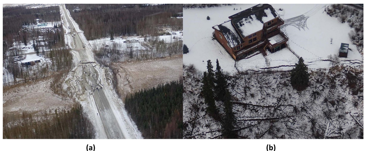
Fig 1. Damage caused by the 2018 Anchorage Alaska earthquake showing (a) lateral spreading along Vine Road close to Wasilla and (b) ground crack propagation along a sloping valley on the south side of Potter Creek in Anchorage.
