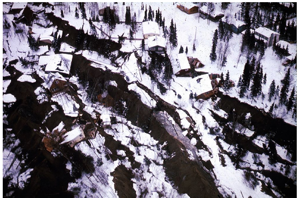
Fig 5. Liquefaction-induced long run-out landslide in Turnagain Heights Anchorage, Alaska generated by the 1964 Great Alaskan Earthquake.
