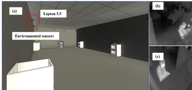
Fig. 6. Hines Hall Artificial Intelligence Laboratory Set Up. (a) 3-D Laboratory layout, analog sensors, and Flir Lepton 3.5. (b) and (c) Thermal images.
