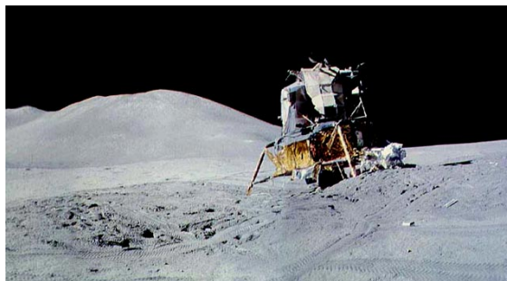
Figure 1: Apollo 15 lander module situated precipitously on the edge of the lunar crater after touchdown due to obscured visibility from the ejecta [12].
