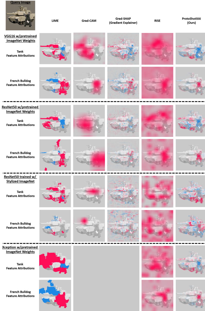
Figure 9: Comparison of feature attributions produced by five different methods (LIME, Grad-CAM, Grad-SHAP, RISE, and ProtoShotXAI) and four different networks. The query image containing the tank and french bulldog is shown in the top left. Each row corresponds to a feature attribution of a given network for a specific class (i.e., tank or french bulldog class). Each column corresponds to a particular approach. Due to the complexity of the Xception Network architecture, the gradient methods, which expect a specific convolutional architecture, were not applicable. The feature attributions from ProtoShotXAI are noticeably more consistent (i.e., positive and negative feature attributions are more isolated to their respective class region).
