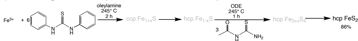
Figure 4. Rational syntheses to six iron sulfides. Grey compounds are presumed and non-isolated intermediates.
