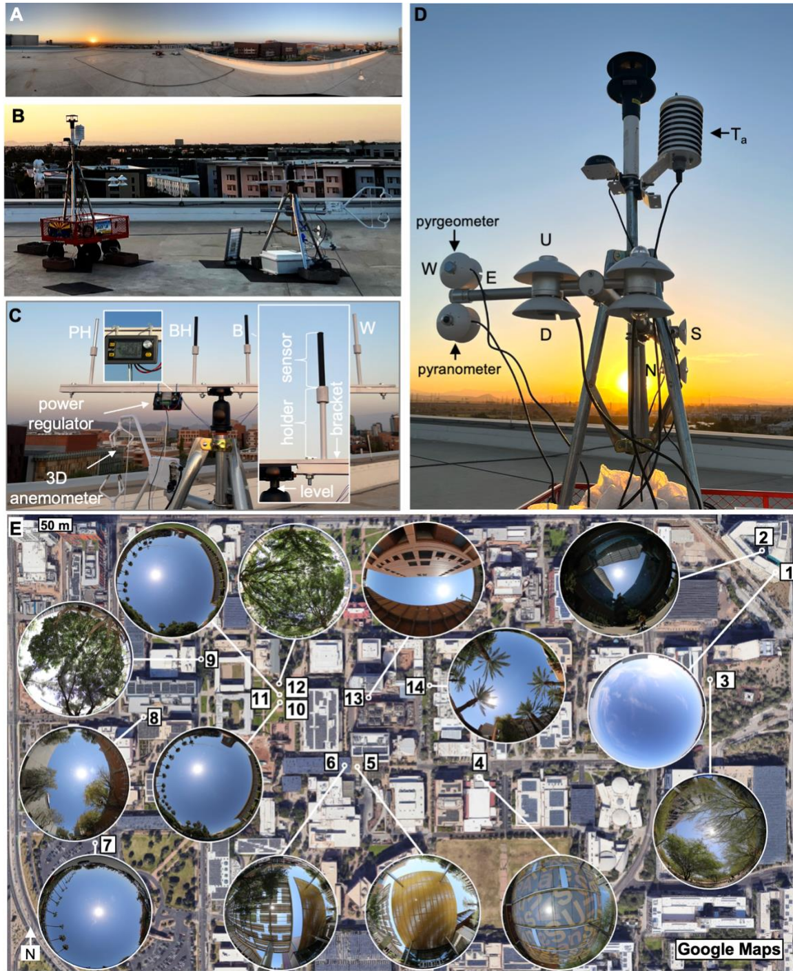
Fig.2 A. and B. The location and sunrise images of the unobstructed view roof site showing placement of MaRTy and tripod (1.5 m apart) with the cylinder array and 3D ultrasonic anemometer; C. close up of the cylinder tripod with marked details, and D. close up of MaRTy with marked details (pyranometer and pyrgeometers face cardinal directions: E-east, W-west, S-south, N-north; facing up-U, facing down-D); E. The location and bottom-up fish-eye images of all the measurement sites in Tempe, Arizona.
