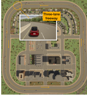
Fig. 4. The example scenario of a 3-lane freeway in CARLA [20]. Vehicles are scattered on the outer loop of the map “Town 05”. The environment is mixed with both autonomous and human-driven vehicles.
