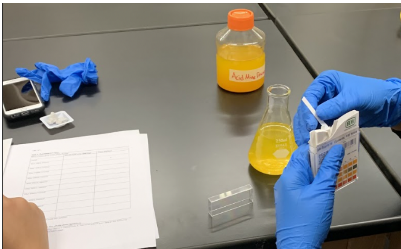
FIGURE 5. Simulated acid mine drainage sample.
