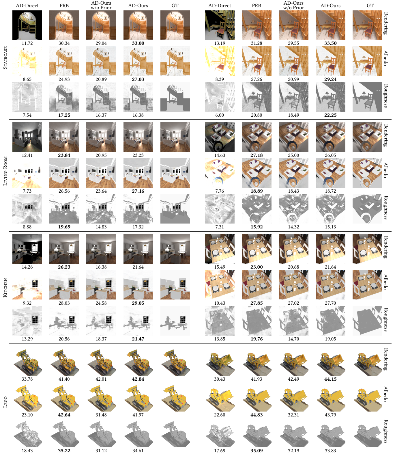
Figure 6: Main results. For each scene, we compare the rendering, recovered albedo, and recovered roughness for direct illumination, PRB, and AD-Ours. We also compare to the case where the radiance cache is trained without the prior. We show two different views of each scene, and report PSNR to ground truth (GT). For STAIRCASE, Ours without prior diverges at 70% progress and we report the best results. Additional scenes are in supplementary.
