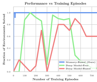
Fig. 3. Agent performance on an unseen computer disassembly environment with respect to number of total training episodes. Our memory-based method converged after 20 episodes.
