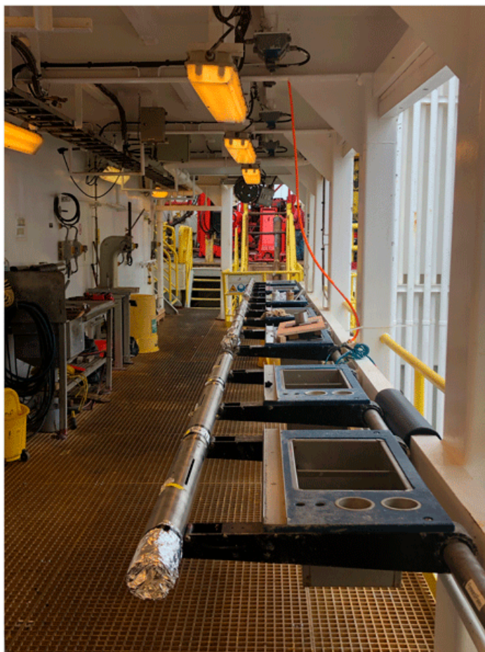
Figure F12. MTFS assembled and ready for deployment on catwalk during IODP Expedition 385T (Wheat et al., 2020).
