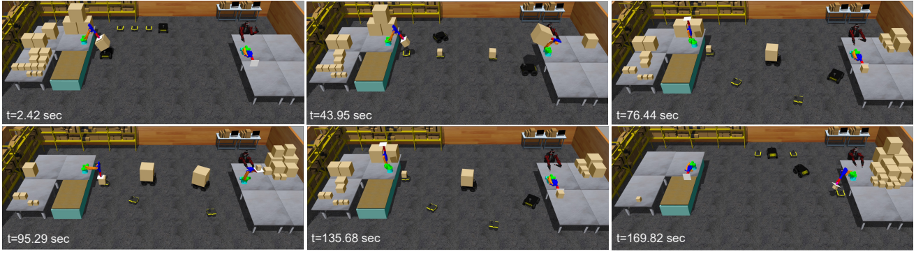
Fig. 3. An example of the qualitative results obtained using Gazebo simulations in ROS to evaluate and demonstrate our method of collaborative scheduling for a team of heterogeneous robots to collaboratively pick and transport a collection of boxes.
