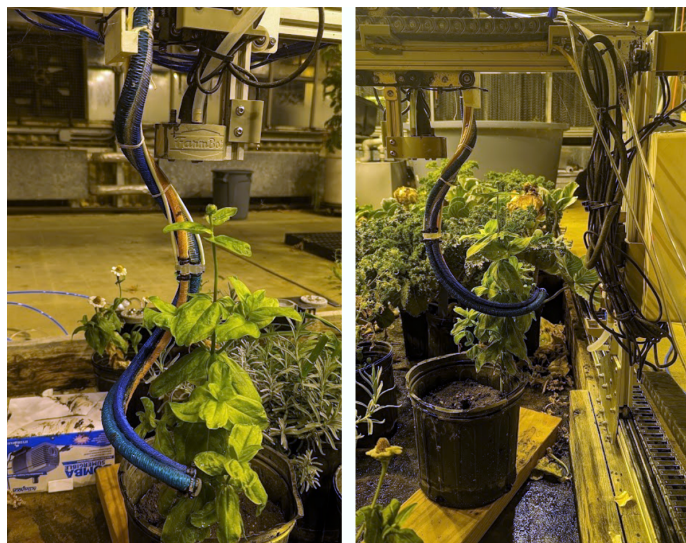
FIGURE 7. BR2-BR2 attached to the FarmBot showing a possible deformation shape to get around the back and under a leaf of a basil plant
