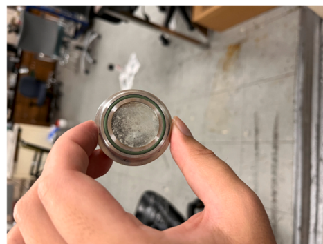
Fig. 4. (left) Testing cell window with minor contamination. (right) Testing cell window with overloaded contaminations.
