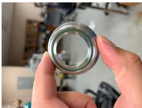
Fig. 4. (left) Testing cell window with minor contamination. (right) Testing cell window with overloaded contaminations.
