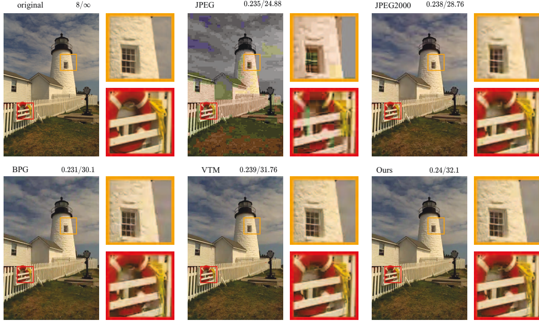
Fig. 9. Visual comparison of our proposed framework with other conventional image codecs, using the bit-rate/distortion [bpp./PSNR \uparrow ] as the metric. The results demonstrate that our method achieves lower distortion in terms of PSNR compared to the other codecs, highlighting its superior capability in preserving image quality.
