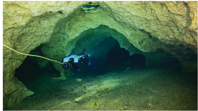
Fig. 1: A BlueROV2 operating inside an underwater cave system by following a caveline ; note that the umbilical is connecting the ROV to a surface operator.
