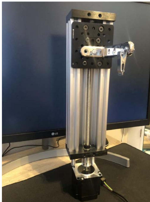
Fig. 7. Assembled linear actuator bundle.
