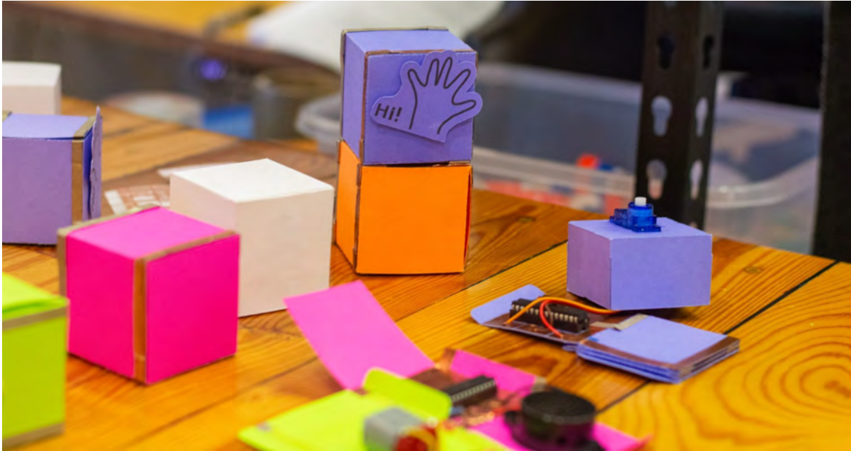
Figure 1: PaBo Bot is a set of modular robots made of colored cardstock paper.
