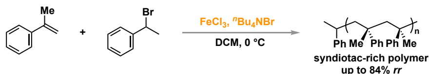
Fig. 59. Stereospecific living cationic polymerization of \alpha -MeSt using \text{FeCl}_3/\text{HBr-St}/n\text{Bu}_4\text{NBr} initiating system [135].
