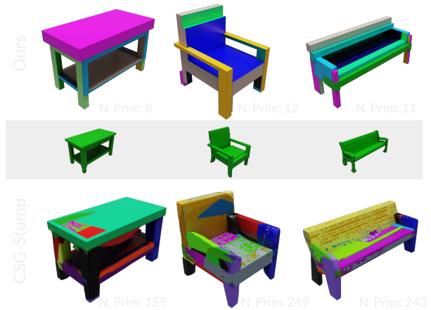
Figure 1. Our method SIRI (top row) generates highly compact yet accurate programs, in contrast to CSG-Stump [24] (bottom row), which generates programs with numerous primitives. Here, we show shapes rendered with colored primitives.
