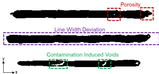
FIGURE 2: EXAMPLE OF THE THREE MAJOR FLAWS OBSERVED IN THIS WORK: POROSITY, DEVIATION IN GEOMETRY OF AN INDIVIDUAL TRACKS (LINE WIDTH VARIATION), AND VOIDS DUE TO CONTAMINATION FROM THE SURROUNDING ENVIRONMENT.
