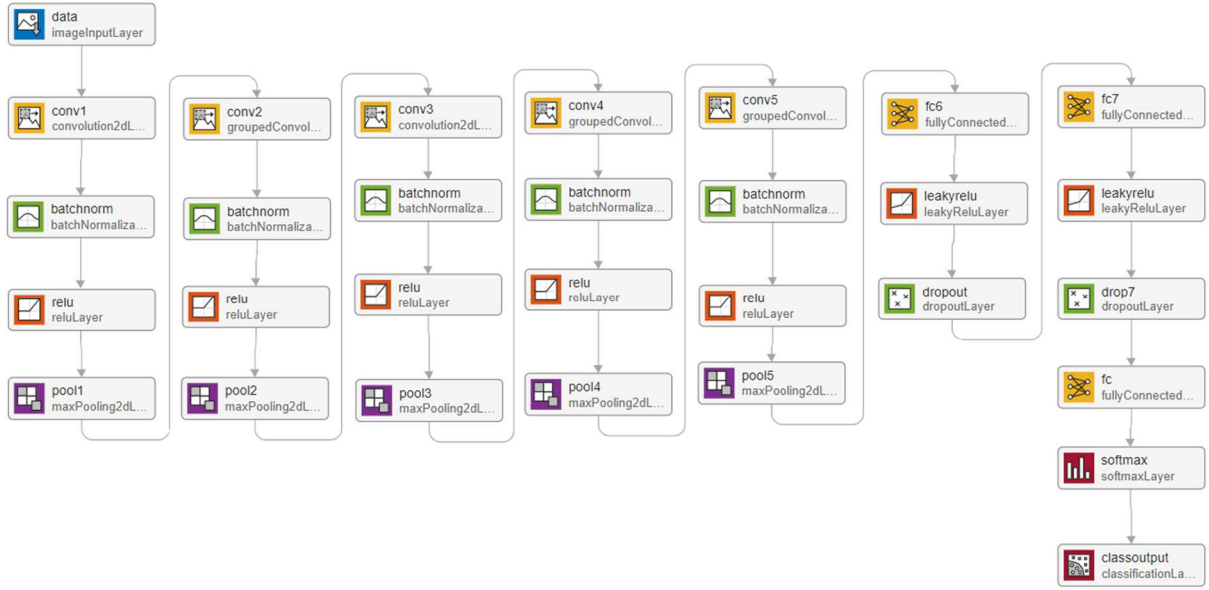
Fig. 4. Proposed Convolutional Neural Network Architecture.
