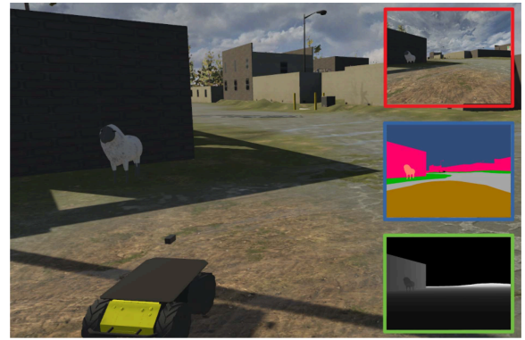
Fig. 1. Robot autonomously explores an unknown environment using an RGBD sensor and a semantic segmentation algorithm.
