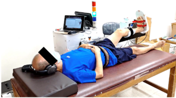
Fig. 5. Practical example of extra-skeletal assisted rehabilitation using a wireless EEG system to monitor brain activity. The system combines a wireless headset with three electrodes and a lower limb rehabilitation robot. The participant used the system to record the changes in lower limb movement and EEG data during the rehabilitation process, and assisted the physician to evaluate the rehabilitation efficacy.
