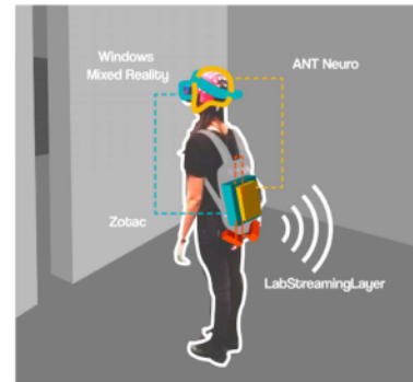
Fig. 6. Example of research by Djebbara et al. [74]. The participants wore a VR head-mounted display (windows mixed reality) on a 64-channel EEG system (eegoSports, ANT Neuro) to study the relationship between cognitive and physical movement.
