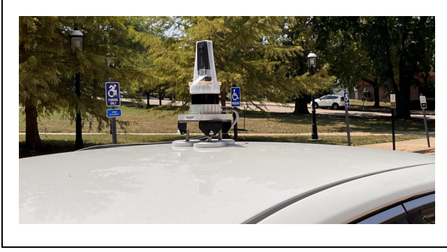
Figure 2. The 360-degree camera-light detection and range (LiDAR) system was assembled and mounted on the top of a vehicle for real-world data collection.
