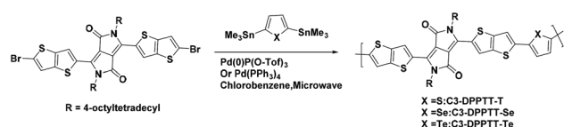
Scheme 6 Synthetic route to chalcogen-containing DPP-TT copolymers.
