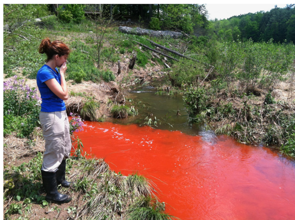
Figure 1. Like most scientists, I don't have a lot of photographic evidence of my failures. But if the chili-pepper red color of this stream and my face don't give it away, this was not the concentration we expected to see downstream during this tracer test.
