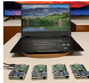
Fig. 10: Raspberry Pi testbed with the laptop working as a server. For SplitGP implementation, the client-side model components are deployed at the Raspberry Pi device, while the server-side model is deployed at the laptop.
