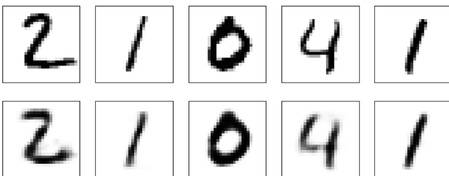
Fig. 6: Top row shows the original input handwritten images, and the bottom row shows the reconstructed handwritten digit images by the configured denoising autoencoder. The structure of the autoencoder is configured such that the binary cross entropy of training and testing is less than 0.1
