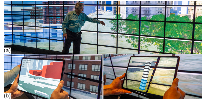
Fig. 8. Interaction with data in the RD can be performed either (a) naturally or (b) using our auxiliary (aux) display system.
