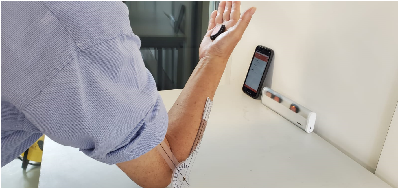
Figure 10. Experimental procedure for angle measurements in two dimensions compared with the angles obtained from the IMU system. The vertical arm of the compass (in white) was fixed onto the lateral side of the upper arm. In contrast, the horizontal arm was mobile to perform accurate 180^\circ amplitude rotations between two segment movements. IMUs and goniometer system coordinates are presented in red and dark grey, respectively. The errors between the two systems are a range of 5% errors.
