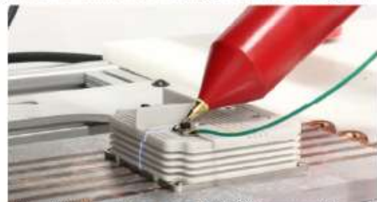
Fig. 10 Surface flashover on a 10 kV SiC power module.
