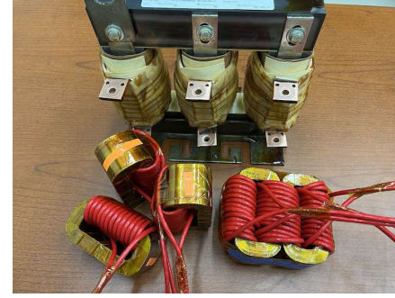
Fig. 14. Inductors used in this study (Upper: TCI V1K130A00; Lower-left: Custom-made separate-cores; Lower-right: Custom-made common-core.)
